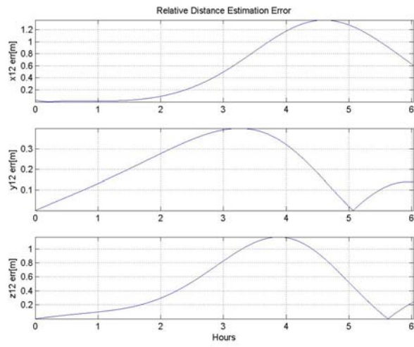
Figure 9: Evolution of the relative position, between the hub and TF 2 , estimation error
