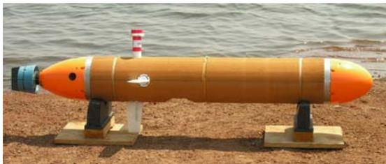
Fig.6 : A photograph of complete Maya AUV
