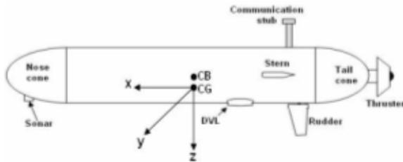
Figure 1: Longitudinal section of the Maya
