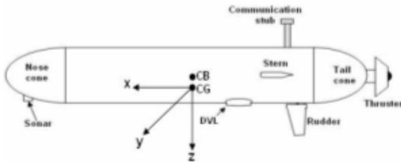
Figure 1: Longitudinal section of the Maya
