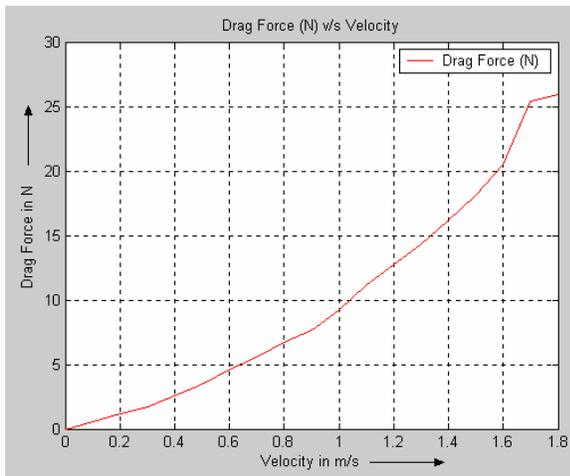
Figure 5: Drag Force (N) against velocity of trolley/AUV
