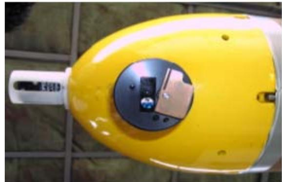
The photograph shows Dissolved Oxygen (DO) sensor mounted on tip of nose cone and the sensing part of chlorophyll-turbidity protruding from the base of the nose cone. A miniature CTD nose cone has also been used with the Maya hull.
