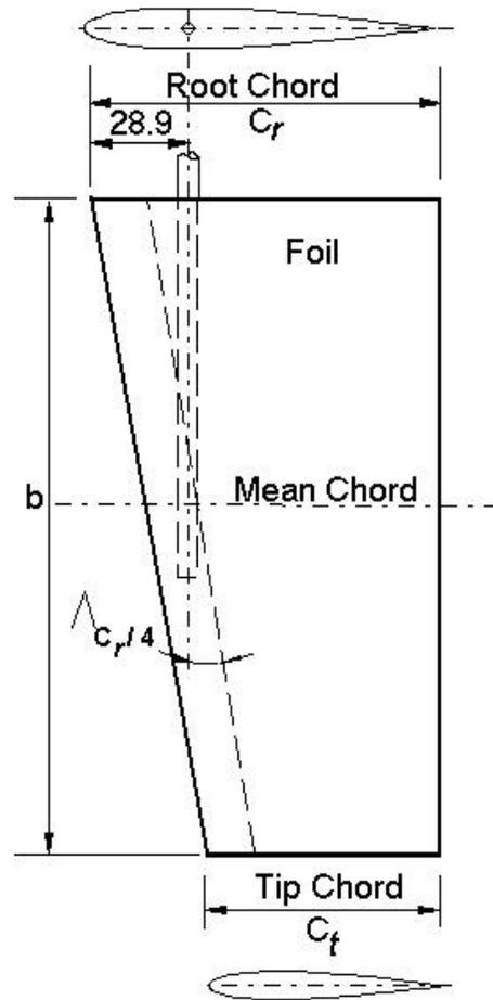
Figure 2: Schematic of control foil on Maya
