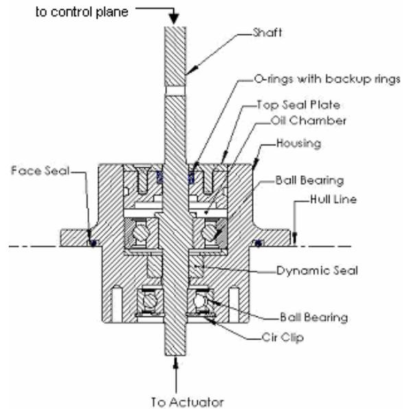
Figure 3: Cross section of shaft seal body
