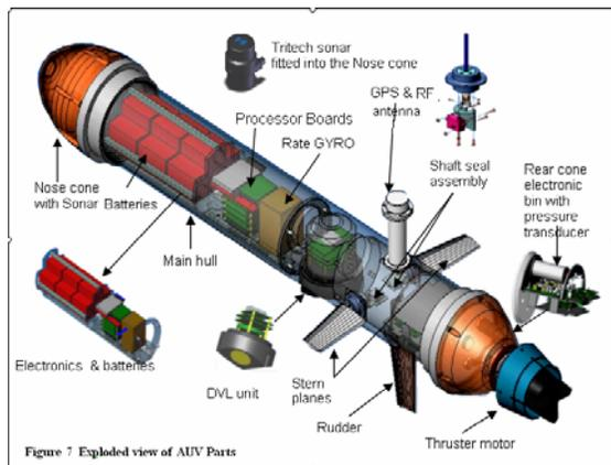
Fig. 7: Solid Works isometric view of Maya.
