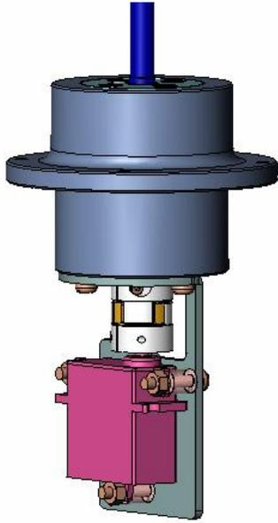
Figure 4: Integrated module of shaft seal with bracket holding coupler and micro-actuator
