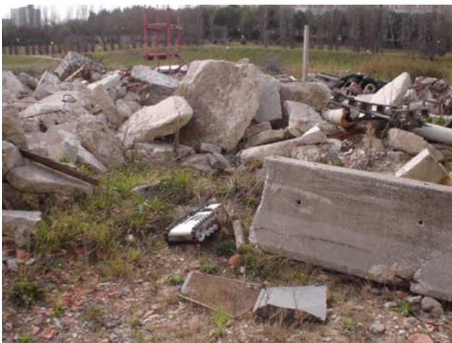
**Figure 12** RAPOSA gets inside a pipe, through a very narrow hole in the rubble
