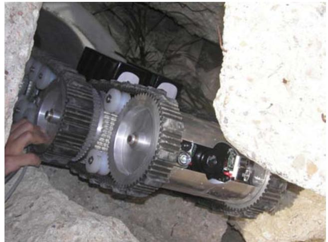
case everything else fails. Figure 8 shows an exercise actually made with the robot, which mimics a standard exercise the Fire Fighters do with their search and rescue dogs, where a person gets inside a hole in the rubble, inside a pipe, and simulates he/she is trapped. The robot was teleoperated and the victim was visible in the infrared cam, as seen in the picture.
