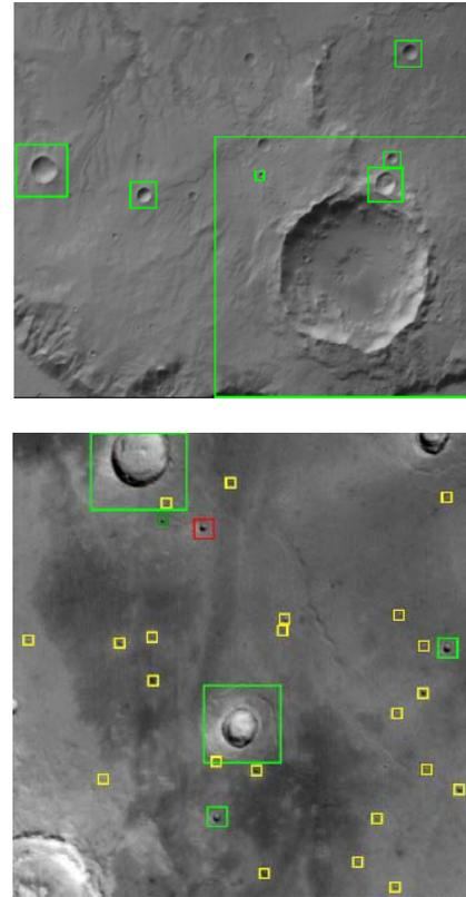
Figure 3 – Output of the classifier: green – correctly classified, red – detection errors, yellow – detection failures in very small craters (below 7 pixels of diameter).
