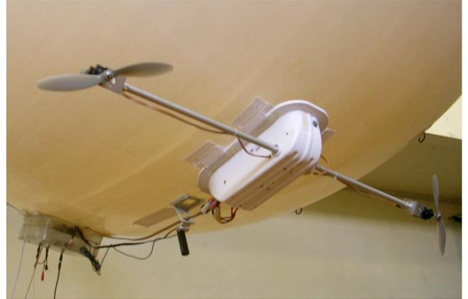
Fig. 3. Underside of the blimp showing the two canopies which contain the hardware and the main propellers.
