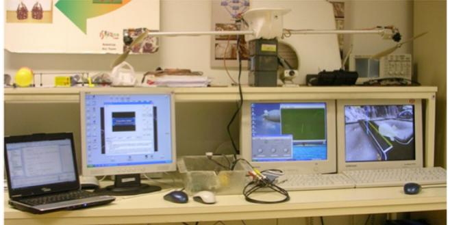
Fig. 7. Picture showing the hardware-in-the-loop simulation setup.
