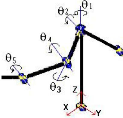
Figure 3: Kinematic model of the human arm.
