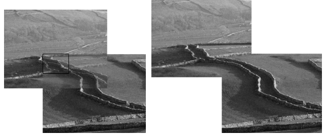
Fig. 3. Registration of images with very small overlap. Left: using a fixed window of size 64 (registration failure). Right: our algorithm.
