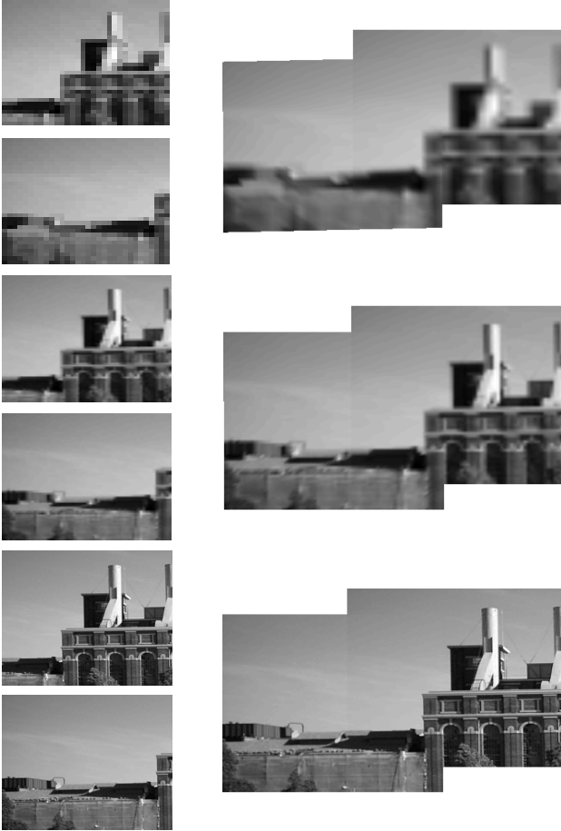
Fig. 5. Three levels of the multiresolution scheme. From top to bottom, the resolution increases. Left column: pairs of images at each resolution level. Right column: registration of the images on the left.
