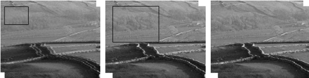
Fig. 2. Registration of a pair of images. Left: using a fixed window of size 64 (registration failure). Middle: fixed window size 128. Right: our algorithm.
