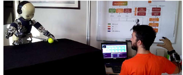
Fig. 1. Experimental setup. The fingers of the iCub robot hand (on the left) are controlled by a human operator with the CyberGlove-II dataglove (on the right).
