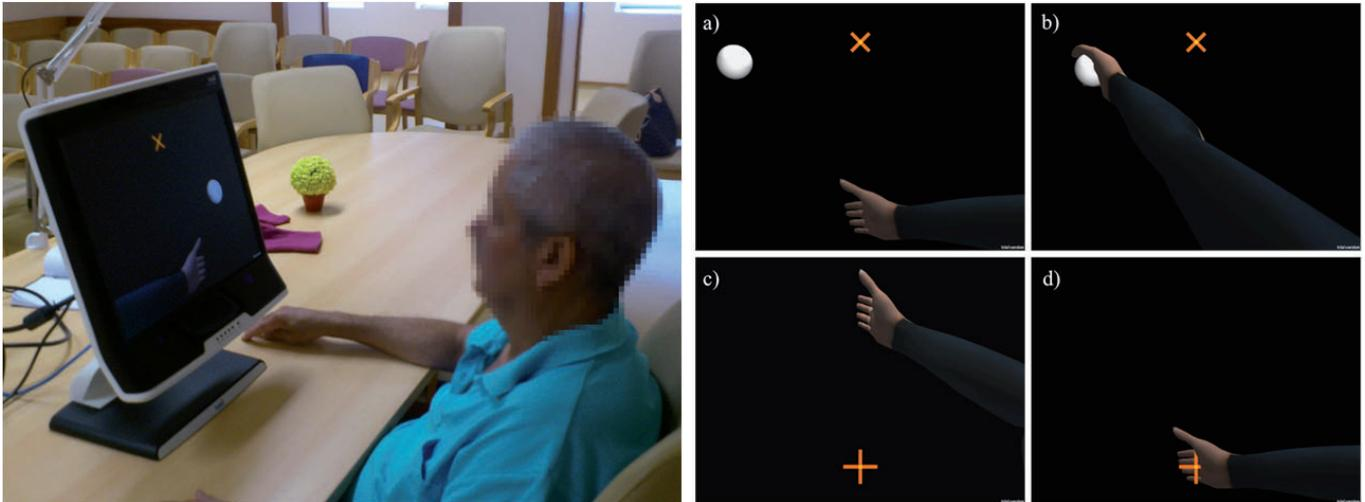
**Figure 1** Experimental setup being used by a stroke patient, consisting of a monitor with an integrated eye tracker running a custom made VR task. The task consist of four steps: a) reaching and grasping of a virtual ball, b) placing it at the target, c) releasing it, and d) moving back to initial position
