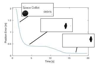
Figure 5: Simulation results for debris scavenging: distance from Space CoBot to the object position, along the three phases explained in the text.
