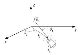
Figure 3: Notation used for modeling a single propeller with respect to the body frame of the robot, centered on its center of mass.
