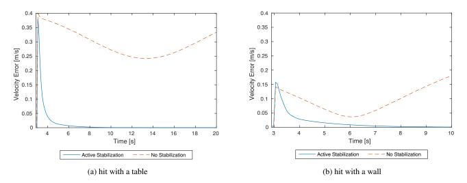
Figure 7: Norm of the linear velocity of Space CoBot, with and without motion stabilization, for the two situations described in the text.
