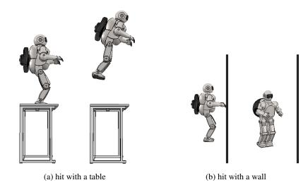
Figure 6: The two simulated situations for the astronaut stabilization task.
