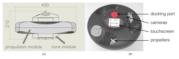
Figure 1: Design of the Space CoBot: (a) side view with the core and propulsion modules indicated with dimensions in millimeters; (b) CAD rendering showing some of the main components.
