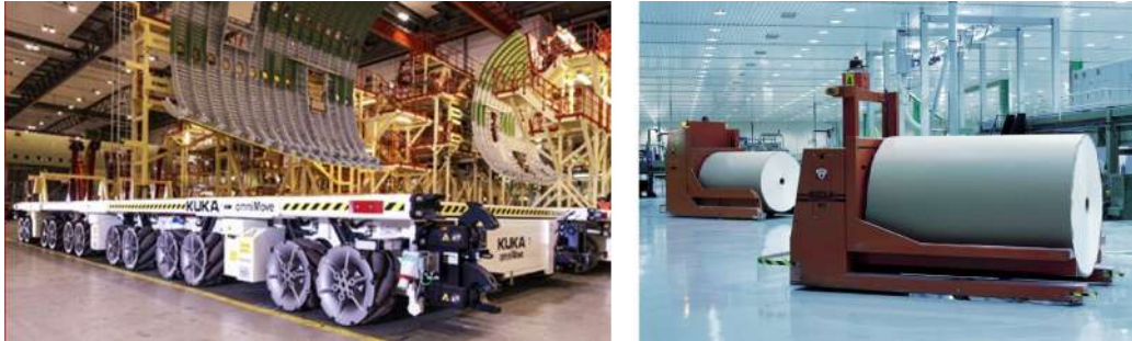
Figure 7: Examples of laser guided vehicles (from left to right): KUKA Industrial Robots ( http://www.kuka-omnimove.com/ ), image obtained from [10], and Efacec AGV to transport paper reels at Soporcel ( http://www.efacec.pt/ ).
