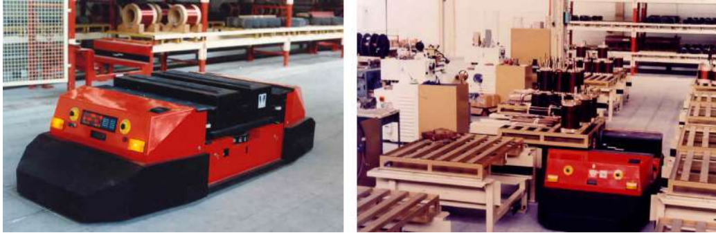
Figure 4: An Automated Guided Vehicle application in industry, the first of its kind in Portugal [1990-1991], with a fleet of four vehicles and wire guidance navigation providing material transportation between 120 operational locations and the two automatic warehouses of Efacec's electrical transformer plant.
