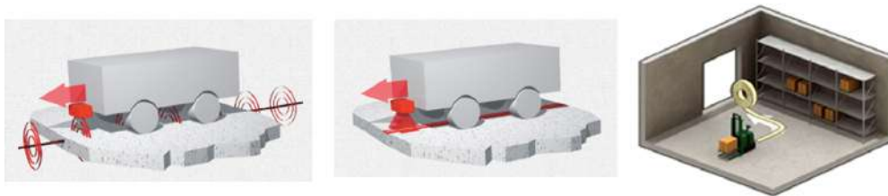
Figure 2: Line guidance principles (from left to right): wire and optical guidance ( http://www.goetting-agv.com/ ) and magnetic tape guidance ( http://www.transbotics.com/ ).
