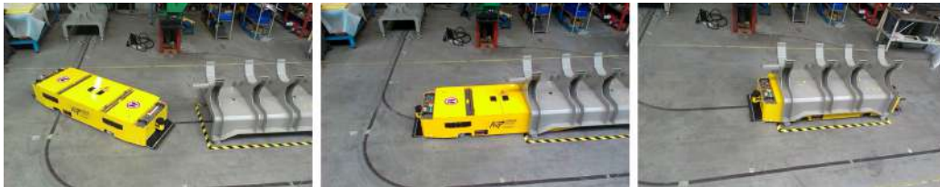
Figure 5: Photos of an AGV designed and build by A-VT Europe NV using line guidance ( http://www.a-vt.be/ ).
