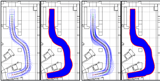
Figure 6: Trajectory to port 1 in equatorial level of TB (from left to right: line guidance and the respective spanned area, free roaming and the respective spanned area).
