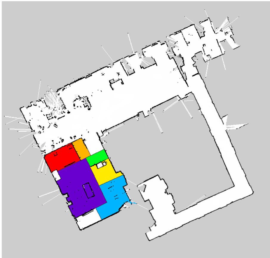
Figure 5.5: Label Map for the Testbed. The map was first obtained with a real robot, and then the labels were drawn.
