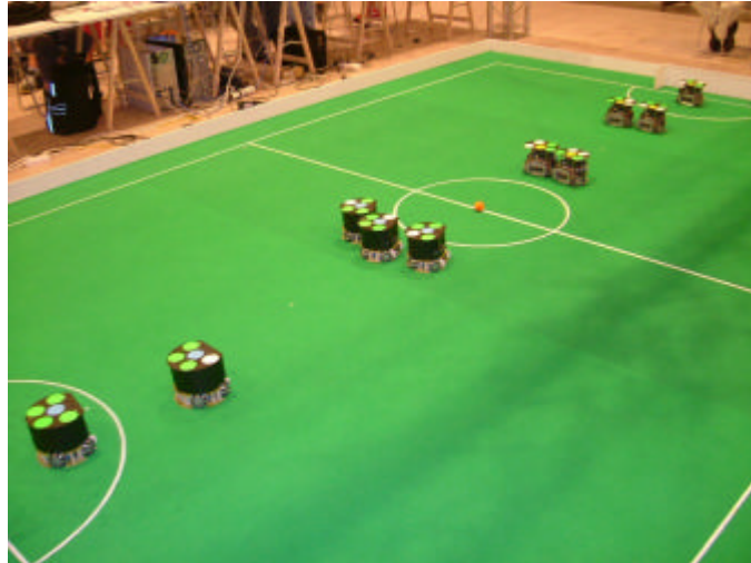
Figure 7: Kick-off during a SSL match. Note the dark shadow cast by the camera mounting structure on the right side of field, which posed a big problem to many teams' vision system
