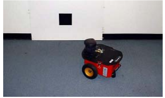
Fig. 1. Experimental setup: Pioneer 2-DXE mobile robot with CCD camera mounted on top and visual landmark.
