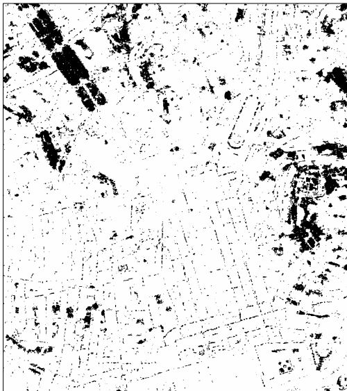
Figure 3. Green color segmentation. Dark areas correspond to regions containing vegetation with high likelihood.
