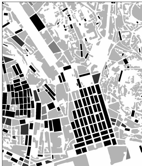
Figure 8. Fitted polygons to all building regions. Rectangular buildings are shown in black, trapezoidal buildings in dark grey and general polygons in light grey.
