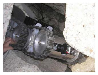
case everything else fails. Figure 8 shows an exercise actually made with the robot, which mimics a standard exercise the Fire Fighters do with their search and rescue dogs, where a person gets inside a hole in the rubble, inside a pipe, and simulates he/she is trapped. The robot was teleoperated and the victim was visible in the infrared cam, as seen in the picture.
