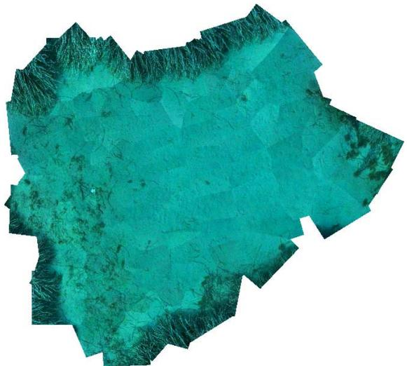
Fig. 3. Final mosaic for the first image sequence. It was created using 129 images selected from the original set of 1000 and rendered with the *closest* operator. The seafloor area covered is approximately  $42 \text{ m}^2$ .
