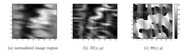
Figure 4.2: Example of gradient magnitude and orientation images
