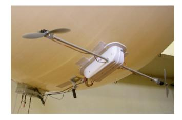
Fig. 3. Underside of the blimp showing the two canopies which contain the hardware and the main propellers.
