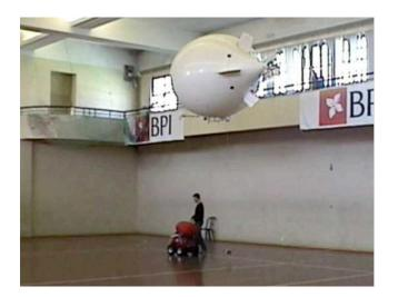
Fig. 15. Real blimp tracking a tele-operated iRobot ATRV-Jr robot.
