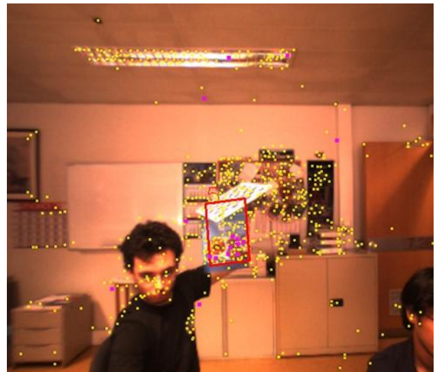
(b) Red: recognized object, yellow: SIFT features, purple: SIFT features matched with the database
