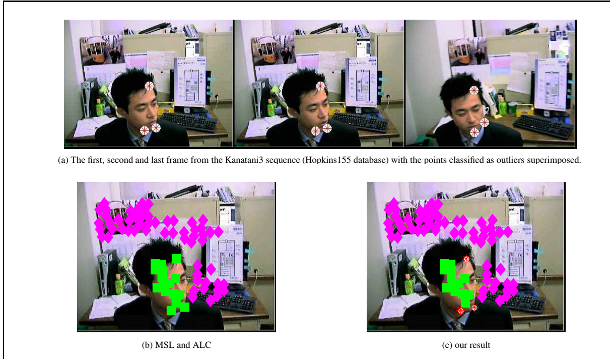
Figure 2. Outlier detection: (a) Feature points in the chin are outliers: their image positions slide along the sequence in a non-rigid way. (b) The segmentation given by the MSL (Sugaya and Kanatani [8]) and ALC (Rao et al. [7]) fails to detect them. Our approach (c) recognizes the outlying trajectories, though admitting one false negative (the forehead point).
