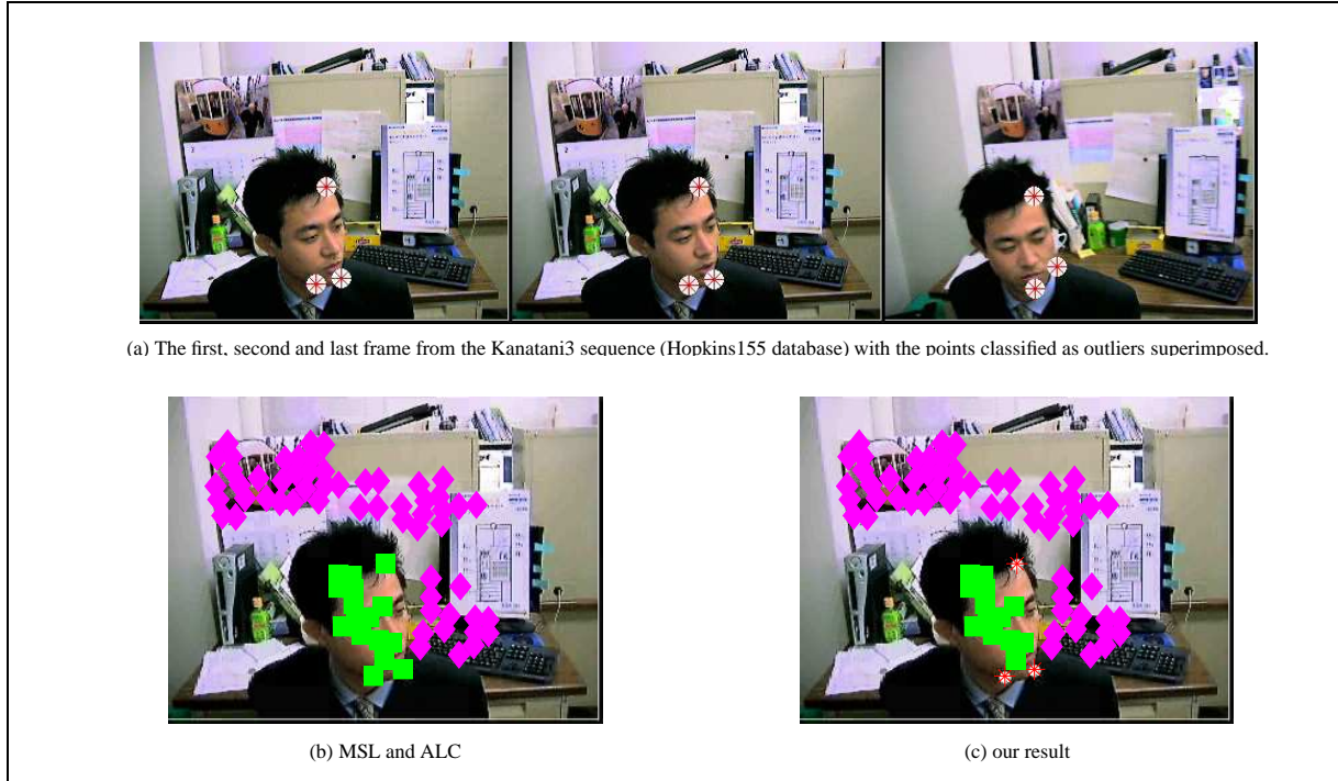
Figure 2. Outlier detection: (a) Feature points in the chin are outliers: their image positions slide along the sequence in a non-rigid way. (b) The segmentation given by the MSL (Sugaya and Kanatani [4]) and ALC (Rao et al. [3]) fails to detect them. Our approach (c) recognizes the outlier trajectories, though admitting one false negative (the forehead point).
