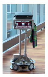
Figure 1: CoBot-2, an omnidirectional mobile robot for indoor users.
