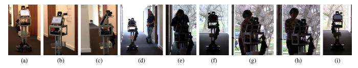
Figure 4: (a,b,c) After CoBot-2 receives a *Transport* task request, it autonomously navigates to the location  $l_p$  to pick up a bottle of water. (d,e) Upon arriving to  $l_p$ , CoBot-2 asks the user to place the bottle of water and press 'Done'. (f,g) Then, CoBot-2 navigates to location  $l_d$  to deliver the bottle of water. (h,i) When the user presses 'Done' CoBot-2 navigates back to its home location. (The complete example sequence is submitted as a video with this paper.)
