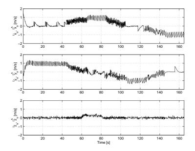
Figure 7.5.6: AUV velocity in the inertial frame  $\{I\}^{\mathcal{I}}\mathbf{v}_{\mathcal{U}} = [{}^{I}\dot{x}_{u}{}^{I}\dot{y}_{u}{}^{I}\dot{z}_{u}]^{T}$  (dashed) and respective estimates  ${}^{I}\dot{x}_{u}, {}^{I}\dot{y}_{u}$  and  ${}^{I}\dot{z}_{u}$ .
