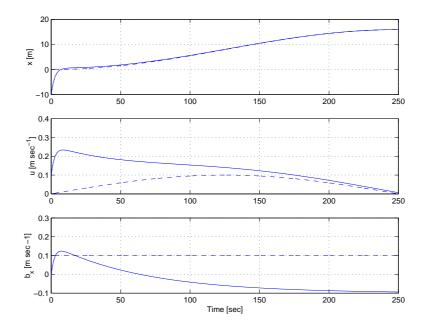
Figure 4.9.8: Position x (dashed line) and position estimate  $\hat{x}$ , on the top; Velocity u (dashed line) and velocity estimate, in the middle and bias  $b_x$  (dashed line) and bias estimate, on the bottom.
