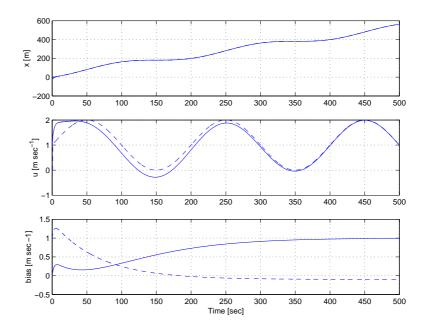
Figure 4.9.14: Position x (dashed line) and position estimate  $\hat{x}$ , on the top; Velocity u (dashed line) and velocity estimate, in the middle and bias  $b_x$  (dashed line) and current estimate  ${}^{I}\hat{u}_w$ , on the bottom.
