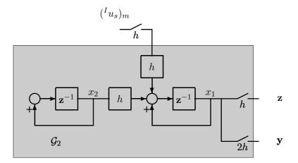
Figure 4.9.3: Position estimation: filter design model.
