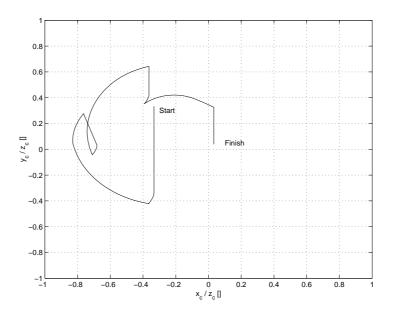
Figure 7.6.3: Camera plane coordinates after compensation for the simulated camera parameters.
