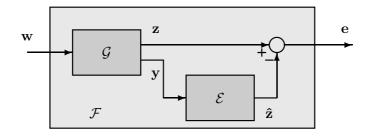
Figure 2.7.1: General setup for filtering synthesis.
