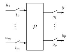
Figure 4.2.1: Multi-rate system with generic sample periods for the inputs and outputs.
