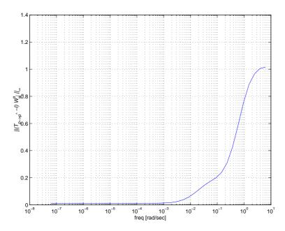
Figure 5.5.2: Analysis of the low-pass operator  $T_{x_m \to \hat{x}}$ . Generalized Bode plot.
