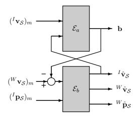
Figure 4.9.13: Block diagram to estimate  ${}^{\mathcal{I}}\hat{\mathbf{v}}_{\mathcal{S}}, {}^{\mathcal{I}}\hat{\mathbf{p}}_{\mathcal{S}}$ , and  ${}^{I}\hat{\mathbf{v}}_{W}$ .
