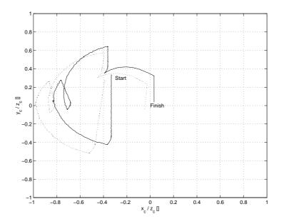
Figure 7.5.4: Camera plane coordinates after compensation for the simulated camera parameters. Exact knowledge of the camera position and orientation in the first experiment (continuous line) and misplaced and misdirected (dashed line).
