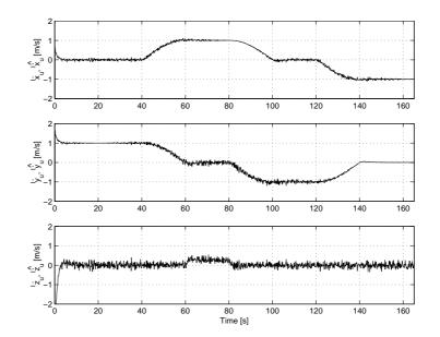
Figure 7.6.2: AUV velocity in the inertial frame  $\{I\}^{\mathcal{I}}\mathbf{v}_{\mathcal{U}} = [{}^{I}\dot{x}_{u}{}^{I}\dot{y}_{u}{}^{I}\dot{z}_{u}]^{T}$  (dashed) and respective estimates  ${}^{I}\dot{x}_{u}, {}^{I}\dot{y}_{u}$  and  ${}^{I}\dot{z}_{u}$ .
