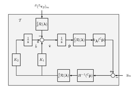
Figure 7.4.1: Non-linear tracker structure.
