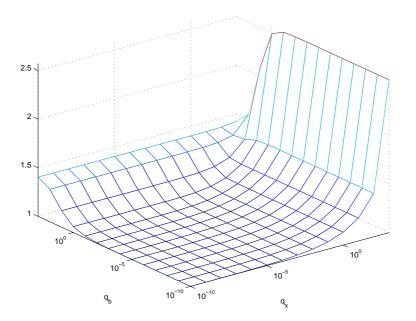
Figure 4.9.4:  $||T_{x_m \to e}||_2$  for a range of  $q_b$  and  $q_x$  values.
