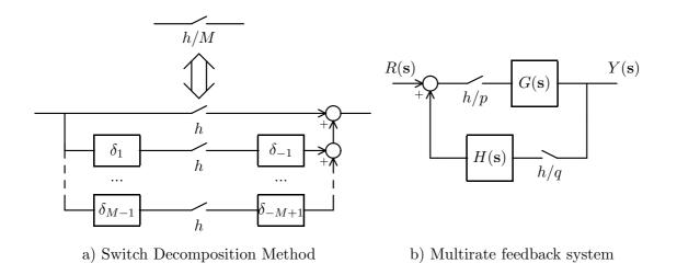
Figure 5.3.1: Multi-rate feedback analysis proposed by Kranc ( $\delta = e^{sh/M}$ ).
