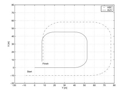
Figure 7.5.1: ASC and AUV inertial coordinates on the horizontal plane.
