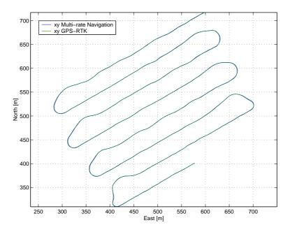
Figure 4.9.9: Trajectory of the Delfim catamaran during a bathymetric survey at sea, in the Setubal canyon.
