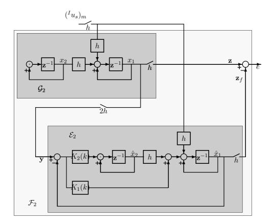
Figure 4.9.7: Estimator design structure for system (4.9.2).
