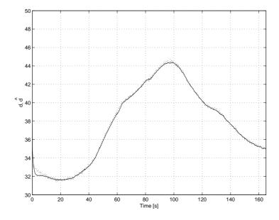
Figure 7.6.4: Distance measured d (dashed) and estimated between both vehicles.
