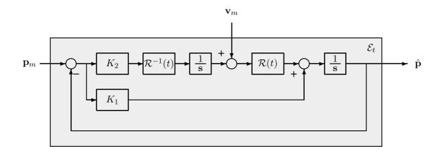
Figure 6.4.1: Non-linear time-varying complementary filter.
