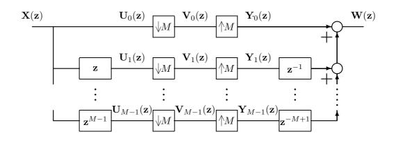
Figure 5.3.2: Digital Decomposition Method.
