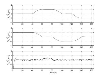
Figure 7.5.3: AUV velocity in the inertial frame  $\{I\}^{\mathcal{I}}\mathbf{v}_{\mathcal{U}} = [{}^{I}\dot{x}_{u}{}^{I}\dot{y}_{u}{}^{I}\dot{z}_{u}]^{T}$  (dashed) and respective estimates  ${}^{I}\dot{x}_{u}, {}^{I}\dot{y}_{u}$  and  ${}^{I}\dot{z}_{u}$ .
