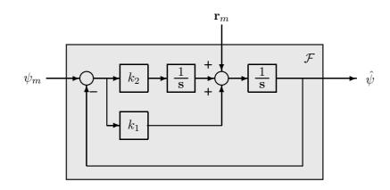
Figure 3.3.3: Complementary filter with bias estimation.
