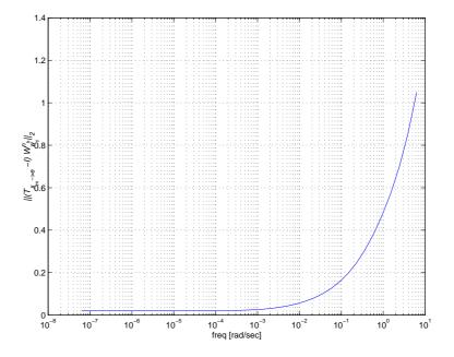
Figure 5.5.1: Analysis of the high-pass operator  $T_{x_m \to e}$ . Generalized Bode plot.
