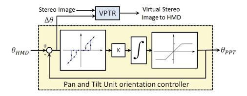
Figure 2.2: Block diagram of the controller.
