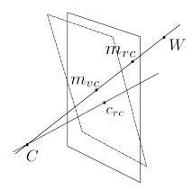
Figure 2.5: Representation of the real camera (rectangle in full line) and the virtual camera (rectangle in dashed line). The virtual camera is a rotation of the real camera over C, the optical center. The indexes rc and vc stand for real camera and virtual camera respectively.
