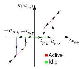
Figure 2.10: Hysteresis transfer function. In red is represented the active mode and in green the idle mode for each angle pan and tilt.
