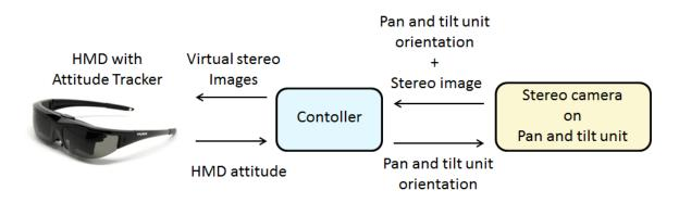
Figure 2.1: System Architecture with the Controller block
