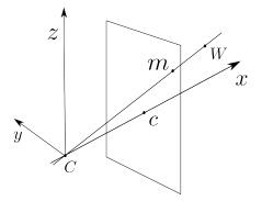
Figure 2.4: Pin Hole camera model
