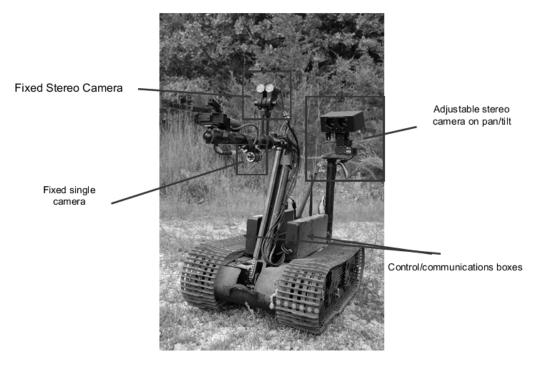
Figure 1.3: U.S. Army TALON robot with additional hardware.
