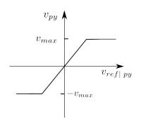
Figure 2.11: Saturation block transfer function.
