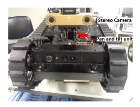
Figure 1.2: RAPOSA-NG with the stereo camera mounted on the Pan and Tilt Unit.
