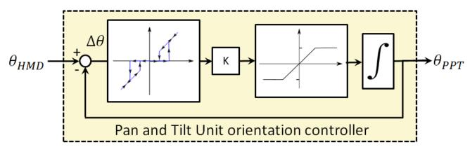
Figure 2.9: Physical pan and tilt controller
