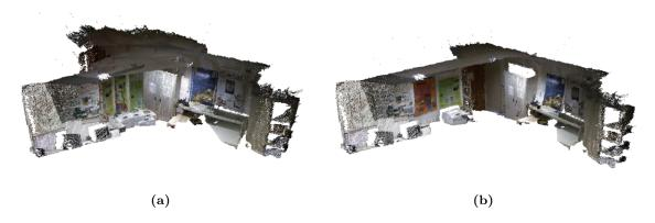
Figure 1.1: (a) Map done using a scan-matching algorithm (see section 2.2) together with a vision-based mapping algorithm (see section 2.3), containing errors in the alignment of some pairs of frames. (b) Map with the alignment between frames corrected using the proposed method presented in this thesis (see chapter 3).
