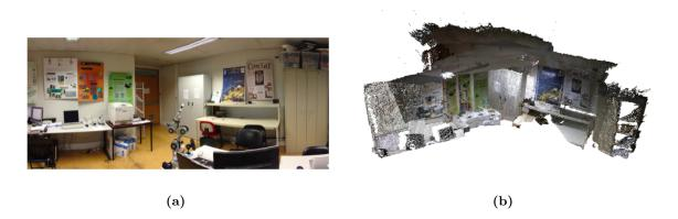
Figure 4.8: (a) Image of the area of the room used to take the dataset. (b) Initial dataset of a map with 15 scans, obtained with Microsof Kinect sensor.
