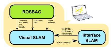
Figure 3.6: Software and Communications Architecture for SLAM using offline data.
