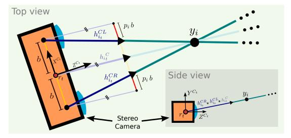
Figure 2.6: Horizontal stereo camera representation.
