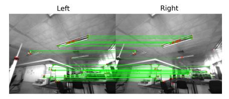
Figure 4.5: Pair of stereo image with visual features. Monocular features are represented with a red dot, while stereo features are represented with a green dot and matched with a green line.
