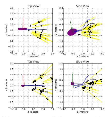
Figure 4.11: SLAM results using DBEKF with different parameters with dataset "B", where G = 0 (top) and G = 1 (bottom). Refer to figure 4.7 for graphical notation.
