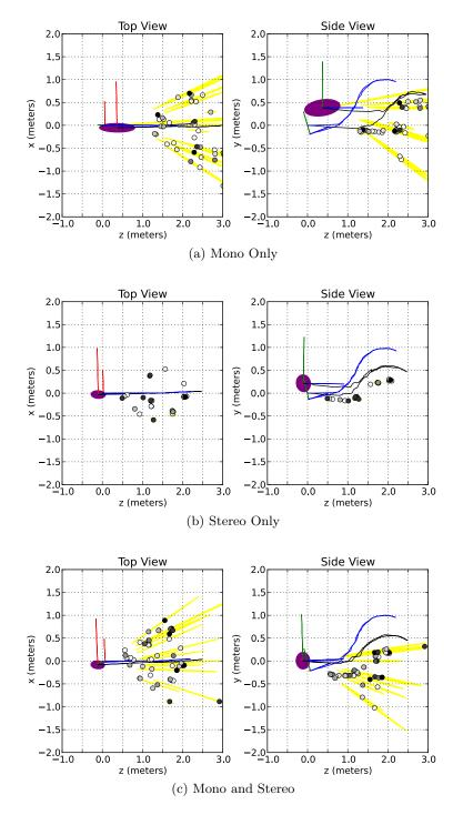
Figure 4.8: SLAM results using DBEKF with dataset "B", using only monocular observations from left camera (a), only stereo observations (b) and both monocular and stereo observations (c). Refer to figure 4.7 for graphical notation.
