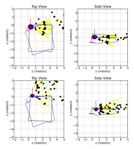
Figure 4.10: SLAM results using DBEKF with different parameters with dataset "A", where G = 0 (top) and G = 1 (bottom). Refer to figure 4.7 for graphical notation.
