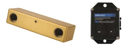
Figure 3.4: Bumblebee  $2^{\textcircled{R}}(\text{left})$  and Microstrain 3DM-GX2R (right)
