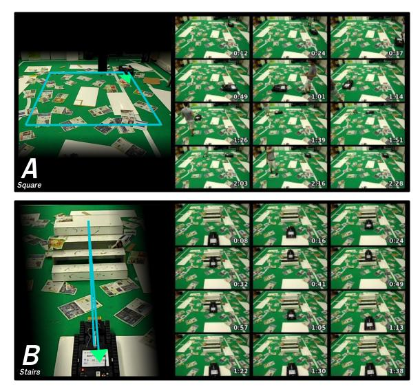
Figure 4.1: Datasets "A" (top) and "B" (bottom). The blue line represents the trajectory travelled by RAPOSA-NG during the experiment, in the direction pointed by the green arrowhead.
