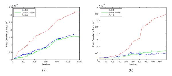
Figure 4.12: Trace of the pose covariance from SLAM using DBEKF with different parameters with dataset "A" (a) and "B" (b).
