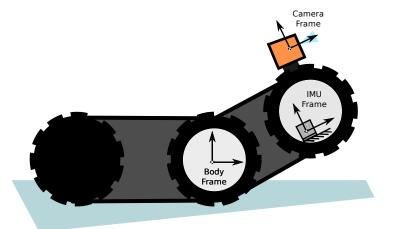
Figure 2.4: A possible Body, IMU and Camera frames configuration for a robot.
