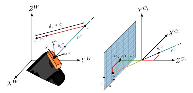
Figure 2.5: Observation Model for landmark  $y_i$ .
