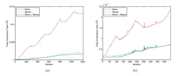
Figure 4.9: Trace of the pose covariance from SLAM using DBEKF for different types of observations with dataset "A" (a) and "B" (b).
