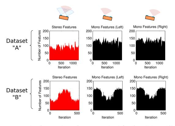
Figure 4.6: Number of stereo and mono features acquired with ORB for each dataset "A" and "B".
