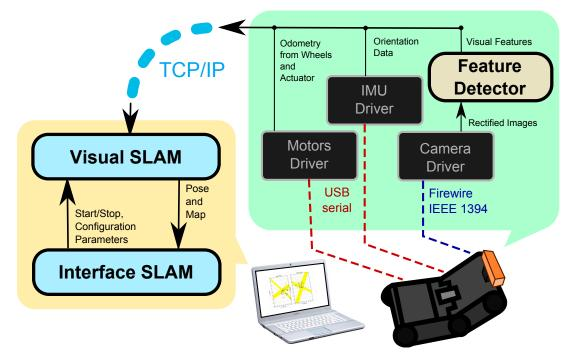
Figure 3.5: Software and Communications Architecture for SLAM on RAPOSA-NG
