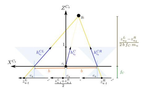
Figure 2.7: Top view of camera frame for stereo vision of a landmark  $y_i$ .
