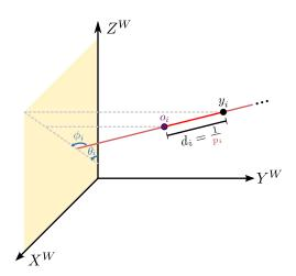
Figure 2.3: Inverse Depth Parametrization for landmark  $y_i$   $(d_i = |y_i^{XYZ} - o_i|)$ .
