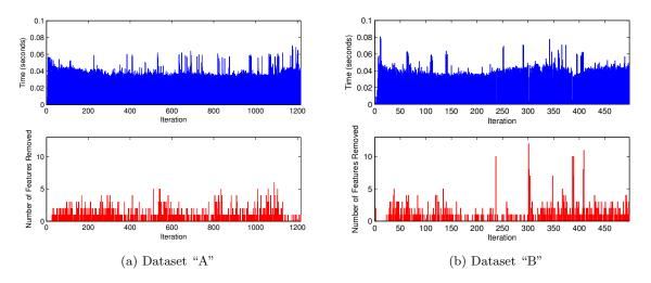
Figure 4.3: Time duration (top) and number of removed features (bottom) per DBEKF iteration for datasets "A" (a) and "B" (b) with both monocular and stereo observations.
