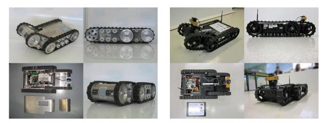
Figure 1.2: Different perspective views and inside view of RAPOSA (Left) and RAPOSA-NG from IST (Right).
