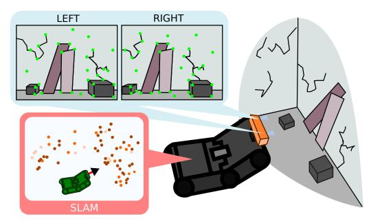
Figure 1.3: Graphical depiction of the proposed SLAM using visual features from a stereo camera.
