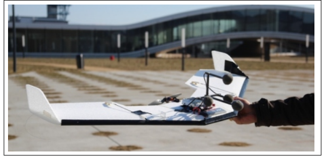
Fig. 5. Picture of the MAV platform [29] used for experimenting the proposed algorithm. Four microphones and an on-board digital sound recorder is used for recording sounds during flight.
