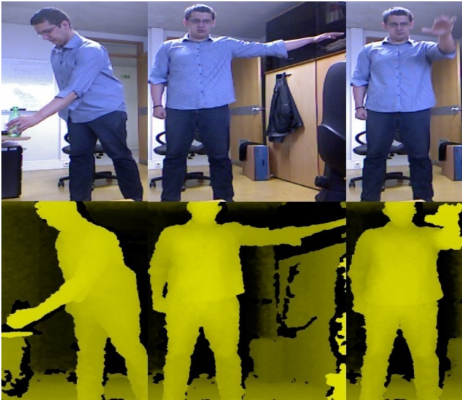
Figure 2: Gesture acquisition using Kinect: RGB (top) and depth (bottom) streams from Kinect
