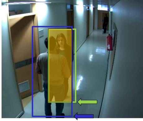
Fig. 4. Example of two overlapping detections and determination of which is occluded. The two Bounding Boxes have a high degree of overlap as shown by the yellow area in the image. In a pair of overlapping detections the one with a higher positioning of its Bounding Box lower boundary (see the arrows) is the occluded one based on geometric considerations. Thus in this image, the woman is heavily occluded.
