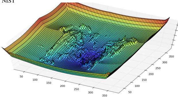
Fig. 9. Energy potential representation of the processed Fig.8 with the goal set at (184, 203) which is the top of a simulated flight of stairs
