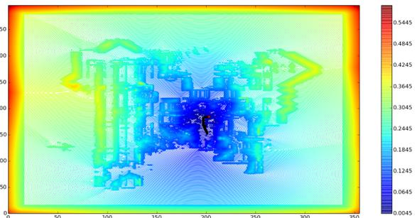
Fig. 12. Path planning over the representation of the isochrone lines of the processed surface represented in Fig.8
