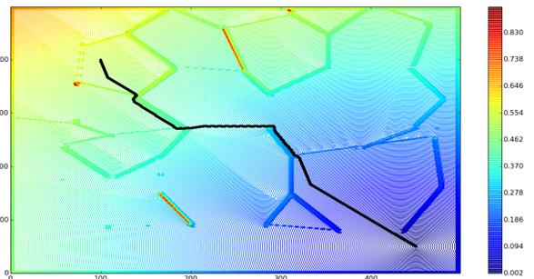
Fig. 11. Path planning over the representation of the isochrone lines of the processed surface represented in Fig.6
