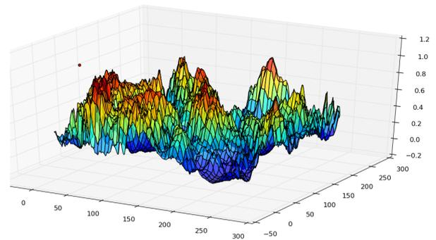
Fig. 4. Rendering of the gray scale elevation map
