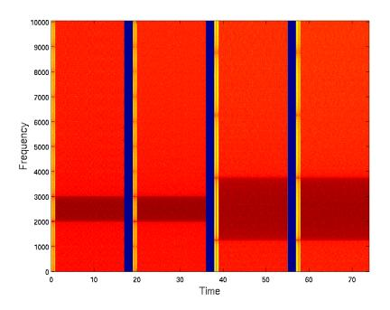
Figure 4.4: spectograms of the transmitted signals: four distinct codes with the same total duration of 1 second of probe signal and 16 seconds of data and then 2 seconds of no signal (blue stripes), giving a total duration of 19 s for each code. Codes are in order A, B, C and D, from left ro right.
