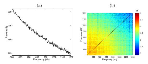
Figure 4.11: Noise spectrum estimated with acoustic data taken at the shallowest hydrophone: periodogram (a) and cross-frequency power spectrum (b).
