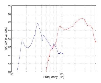
Figure 4.1: Transmitting source frequency response.
