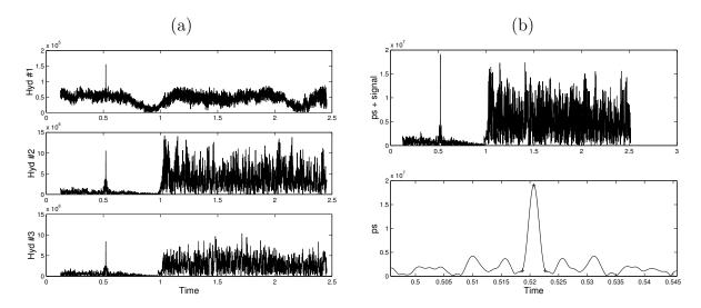
Figure 4.13: virtual time reversing of the received code B for hydrophones 1, 2 and 3 (a) and summation of the time reversed data of hydrophones 1, 2 and 3 [upper plot of (b)] and detail of the probe signal pulse shape [lower plot of (b)].
