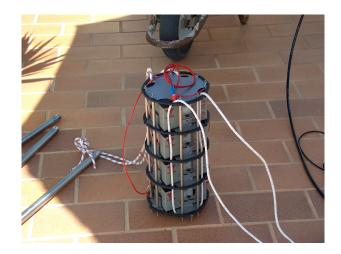
Figure 2.5: Acoustic Oceanographic Buoy battery pack.
