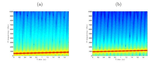
Figure 4.2: Transmitted LFM signals: lower band 400–900 Hz (a) and upper band 900–1300 Hz (b).
