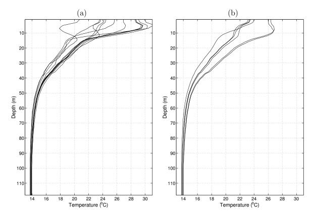
Figure 4.8: Acoustic inversion for ocean temperature during day June 21st, with signals in the band: (a) 500-800 Hz; (b) 900-1200 Hz.
