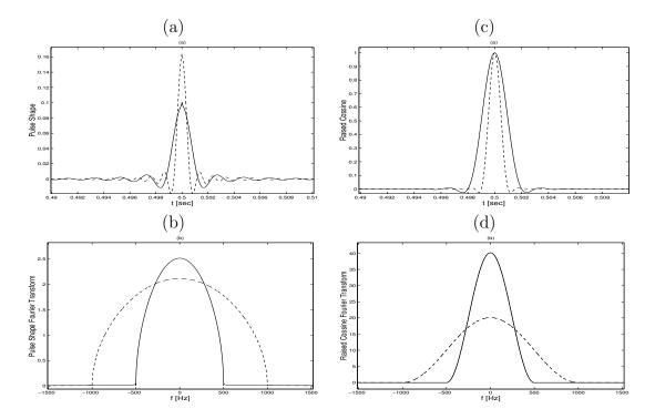
Figure 4.3: pulse shape: root-root raised cosine (a) and its spectrum (b), root-raised cosine (c) and its spectrum (d); continous line is for 500 symbols/s while the dashed line is for 1000 symbols/s.
