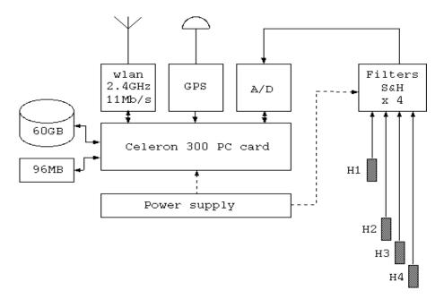
Figure 2.1: Acoustic Oceanographic Buoy - version 0: block scheme.
