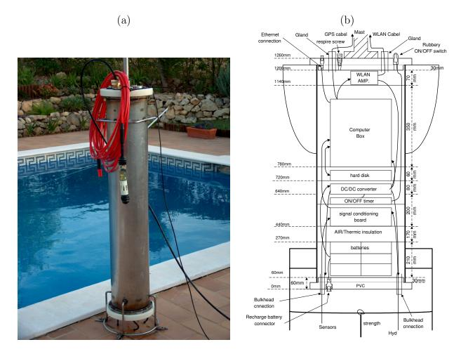
Figure 2.2: Acoustic Oceanographic Buoy (AOB): picture during preliminary swiming pool testing (a) and internal configuration (b).
