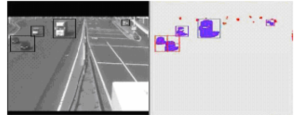
Fig 4. Tracking and occlusion handling on highway
