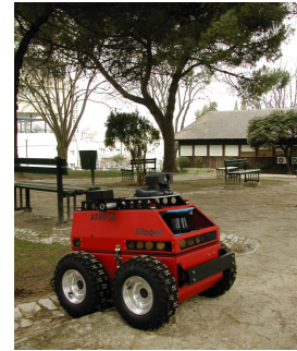
Fig. 6. Mobile Robot ATRV-Jr with a Pan and Tilt camera Sony EVI-D31
