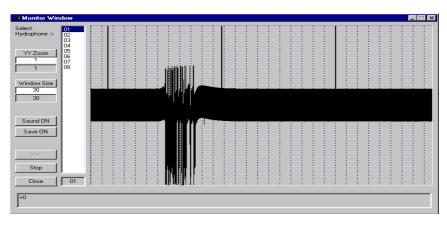
Figure 2: Monitor window to visualize the data being acquired at the remote buoy.
