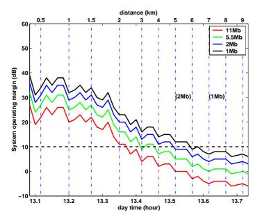
**Figure 3:** Measured system-operating margin of the wireless communication sub system between buoy and the ship during the sea trial test, with the omnidirectional antenna. Dashed line at 10 dB is the WLAN manufacturer requirements for a "good connection". Values within parenthesis are the real throughputs achieved at given time/distance (only worst case values represented).
