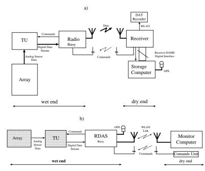
**Figure 1**: Block schema of the Ultra Light Vertical Array (ULVA) : original layout (a); modified ULVA with the remote data acquisition system (RDAS) (b), original blocks are shadowed.
