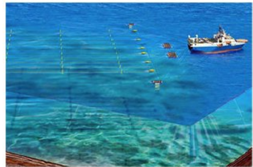
Figure 1: Conventional geophysical surveying using long lines of towed streamers
