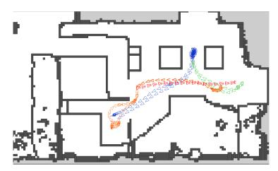
Figure 4.33: Representation of the robot path while executing the new patrol task.
