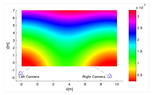
Figure 3.6: Variance as function of the position of the measurement.
