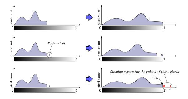
Figure 2.5: Examples of the effect of the Max-RGB algorithm on the histogram.
