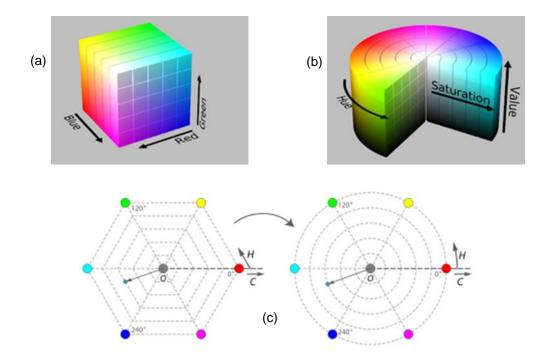
Figure 2.1: (a) RGB color space; (b) HSV color space; (c) Morphing of hexagon in chromaticity plane. Images by Jacob Rus used under CC BY license.
