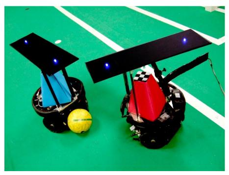
Figure 3.1: MSL robots with tracking marker apparatus.
