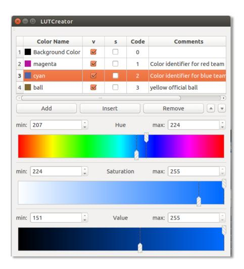
Figure 2.4: LUTCreator control panel.
