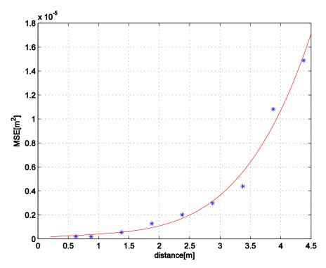
Figure 4.4: Estimate of the ground plane position measurement error variance as a function of distance.
