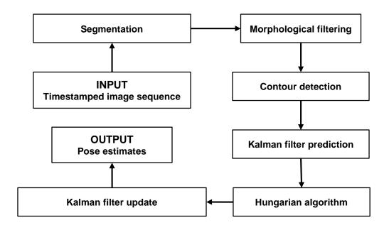
Figure 3.7: Sequence of processing operations.
