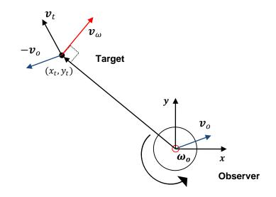
Figure 5.1: Obstacle velocity components.
