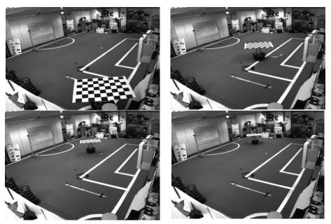
Figure 3.3: examples of checkerboard images used to estimate the error variance.
