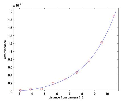
Figure 3.5: Variance as a function of the distance from the camera.
