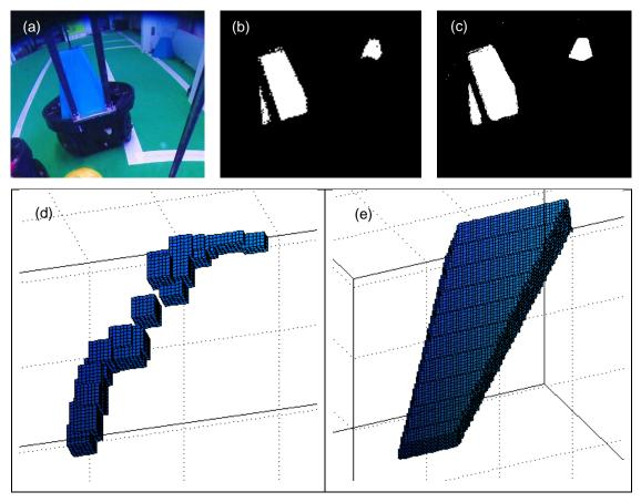
Figure 2.2: (a) Raw image ; (b) binary image resulting from the RBG picking method; (c) binary image resulting from the HSV intervals ; (d) LUT produced with the RBG picking method; (e) LUT produced by HSV intervals.
