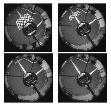
Figure 4.2: A few of the images used for estimation of error variance, patterns at distances of 25cm, 100cm, 250cm and 400cm.
