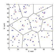
Figure 9.5: Static targets final synchronous-distributed partition (quadrotors, fixed-wings).
