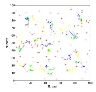
Figure 9.10: Slow targets quadrotors path: the red crosses represent the targets final positions and the coloured lines the agents path obtained with the algorithms of Figure 9.8.
