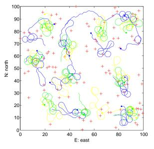
Figure 9.18: Fast targets fixed-wings path: the red crosses represent the targets final positions and the coloured lines the agents path obtained with the algorithms of Figure 9.16.
