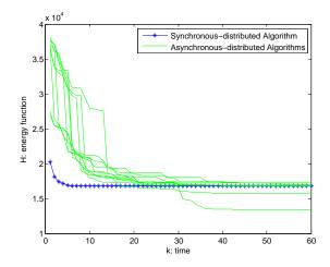
Figure 6.5: Asynchronous-distributed coverage algorithm: convergence to synchronous-distributed solution.
