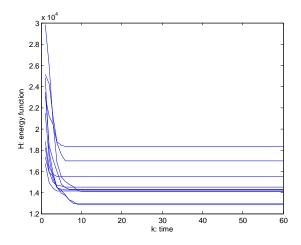
Figure 6.4: Synchronous-distributed coverage algorithm: many local minima.
