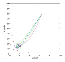
Figure 7.7: Fixed-wing linearised local tracking SCP paths: the red crosses represent the targets final positions and the coloured lines the agent path obtained with different SCP parameters.
