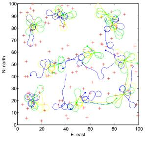
Figure 9.4: Static targets fixed-wings path: the red crosses represent the targets final positions and the coloured lines the agents path obtained with the algorithms of Figure 9.2.
