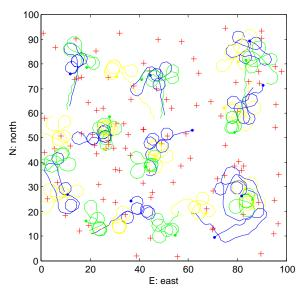
Figure 9.11: Slow targets fixed-wings path: the red crosses represent the targets final positions and the coloured lines the agents path obtained with the algorithms of Figure 9.9.
