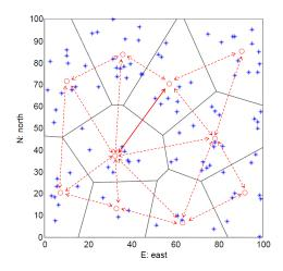
Figure 6.3: Asynchronous-distributed Algorithm 2 where only a random pair of neighbour agents communicate at each time-step.
