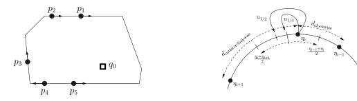
Figure 3.4: Sensors placed along a static boundary surrounding the target (from Martínez and Bullo [33]).
