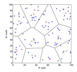
Figure 6.1: Partition example for solving agent-target assignment problem. The red circles represent the position of the agents and the blue stars the position of the targets.
