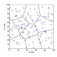
Figure 9.12: Slow targets final synchronous-distributed partition (quadrotors, fixed-wings).
