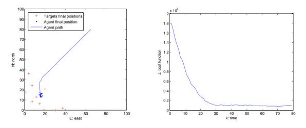
Figure 7.3: Quadrotor local SDP path.
