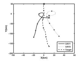
Figure 3.3: Fixed-wing tracking behaviour (from Zhan et al. [54]).
