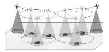
Figure 1.1: Multi-UAV Multi-Target Tracking (from Tang and Ozguner [51]).
