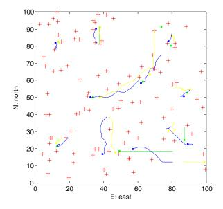
Figure 9.3: Static targets quadrotors path: the red crosses represent the targets final positions and the coloured lines the agents path obtained with the algorithms of Figure 9.1.
