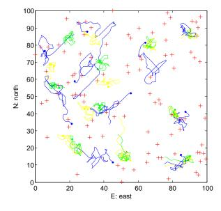
Figure 9.17: Fast targets quadrotors path: the red crosses represent the targets final positions and the coloured lines the agents path obtained with the algorithms of Figure 9.15.
