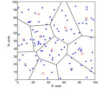
Figure 9.13: Slow targets final asynchronous-distributed partition (quadrotors).
