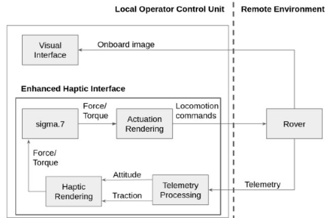
Figure 5. System architecture for the proposed teleoperation interface.
