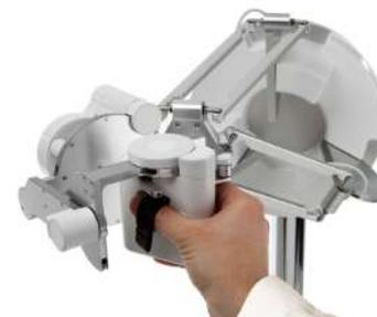
Figure 3. Operator holding the 7-DOF haptic input device sigma.7 from Force Dimension<sup>1</sup>.
